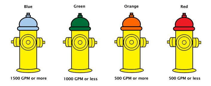
Each fire hydrant should be capable of delivering a flow of at least 500 gallons per minute with a residual pressure of not less than 20 psi.
